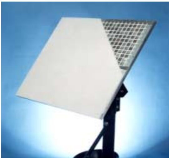
Figure 1. Dual-Polarized Ku-Band CTS Array Figure 2. Measured Pattern for Dual-Polarized CTS Array
