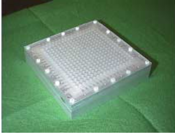
Figure 3. Dual-Polarized/Dual-Band CTS Array
